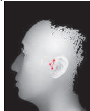
Fig.1 Three Points Used For Plane Fitting
