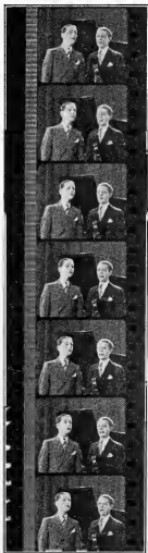
Phonofilm—actual size, the sound track showing to the left of the action photographs. This actual recording shows a continuous sound—that of a male duet with a musical accompaniment. On cessation of sound the sound track shows absolutely black on the positive prints.
