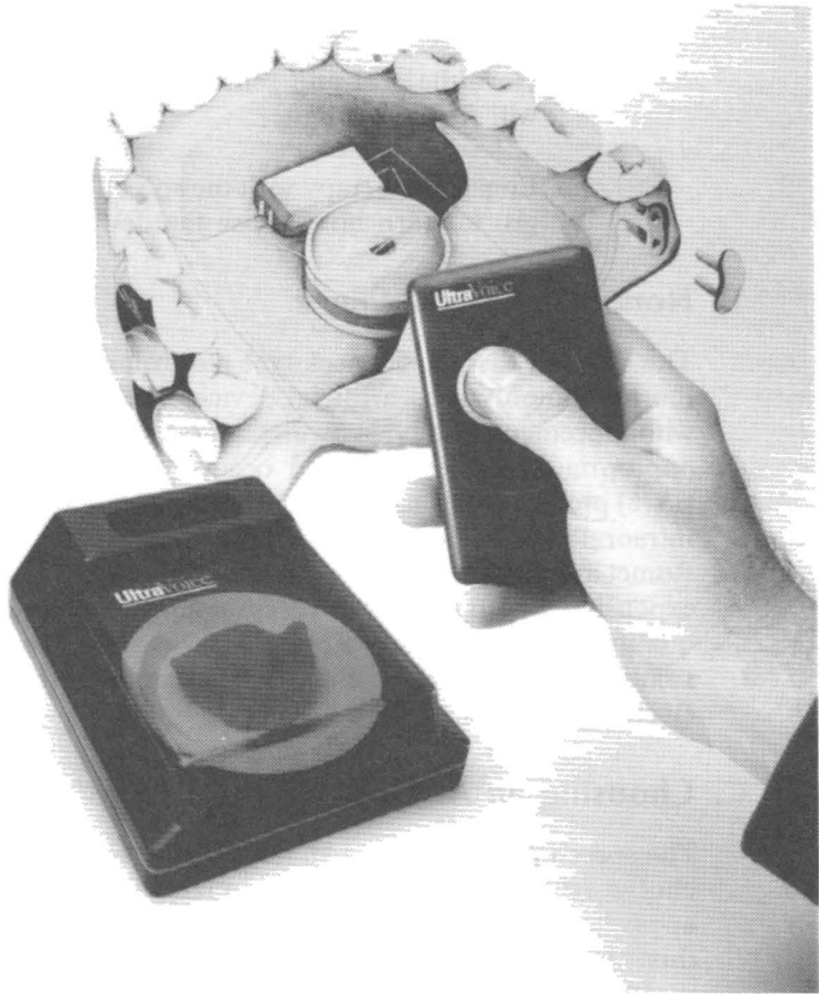
Figure 5-5. Picture of Ultra Voice device showing components mounted into an upper denture and hand held remote control unit with chargers. (Available from Health Concepts, Inc., 279-B Great Valley Parkway, Malvern, PA 19355. Phone [800] 673-7881.)
