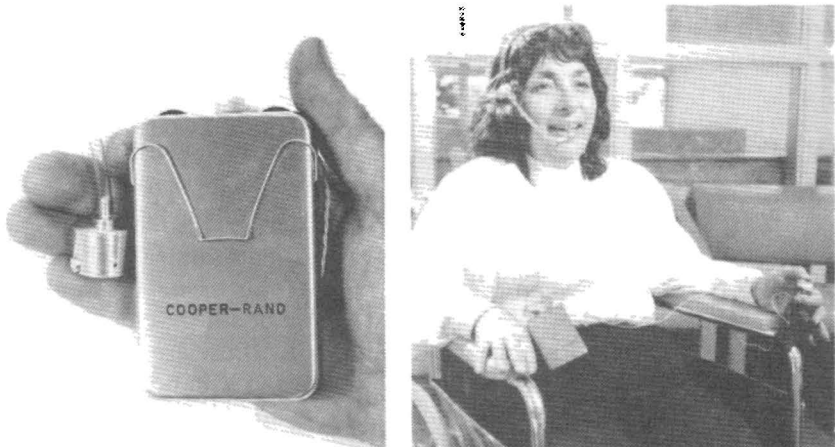
Figure 5-4. Picture of the Cooper-Rand intraoral artificial larynx which can also be adapted for use by wheelchair-bound patients or patients with the need for hands-free activation. (Available from Luminaud, Inc., 8688 Tyler Blvd., Mentor, OH 44060. Phone: [216] 255-9082.)
