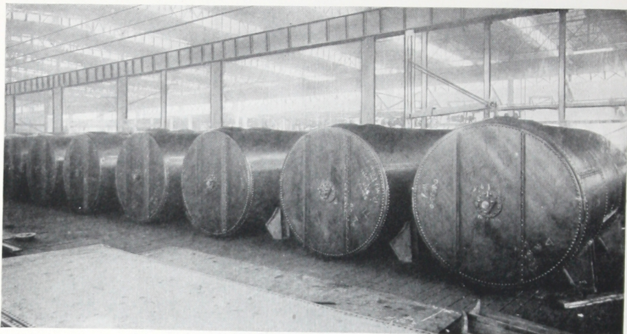
Part of a Series of Sugar Crystallizers Furnished United Fruit Co., Cuba
